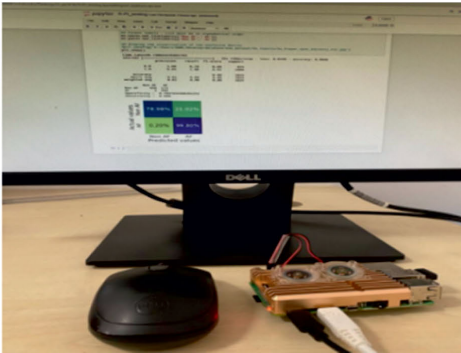
Fig. 1. Implementation of the proposed optimal convolutional neural network models on resource constrained computing platform (Edge computing): Raspberry-Pi computing platform with Broadcom BCM2711 and 1.5 GHz Cortex-A72 quad-core CPU with 8 GB RAM
